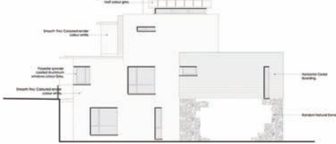
ELEVATION 4 SIDE ELEVATION (NORTH EAST)
