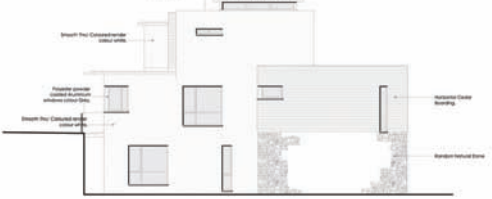
ELEVATION 4 SIDE ELEVATION (NORTH EAST)
