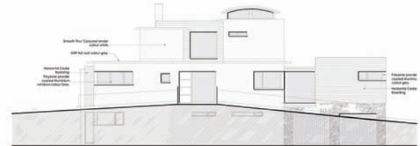
ELEVATION 3 REAR ELEVATION (SOUTH EAST)
