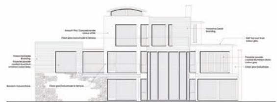
ELEVATION 1 FRONT ELEVATION (NORTH WEST)
